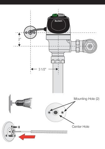
Drill two (2) mounting holes into wall and mount flange using the appropriate fasteners for the particular wall type.
