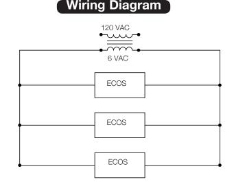
One EL-386 Transformer serves one (1) Optima Closet/Urinal Flushometer. One EL-451 Transformer serves up to six (6) Optima Closet/Urinal Flushomteres. 18 gauge wire (not supplied) required from transformer to flushometers.
