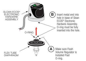
C Push Diaphragm securely against underside of Sloan ECOS® Electronic Assembly. Place entire Assembly onto the Valve Body.
